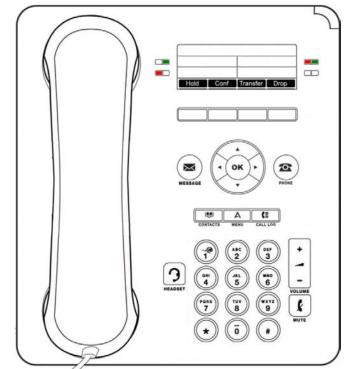
The phone supports 12 programmable call appearance/feature buttons. The labels for these are displayed in the main display and can be controlled by the adjacent buttons.
