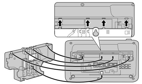
Fasten the wall mounting adaptor to the base with 1 screw. (Recommended torque: 0.4 N⋅m [4.08 kgf⋅cm/ 3.54 lbf⋅in] to 0.6 N⋅m [6.12 kgf⋅cm/5.31 lbf⋅in])
