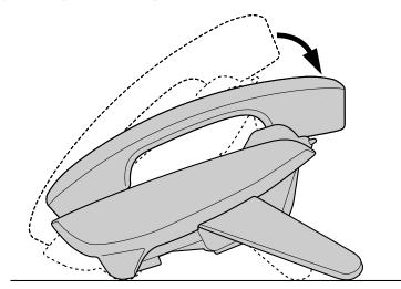
1. Tilt the stand in the direction indicated while pushing the PUSH mark with both hands as shown until it locks into the low position (**B**).
